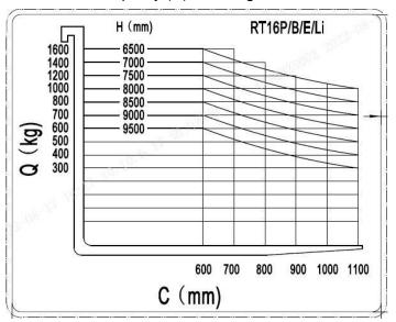
Fig. 10: Residual lift diagram
