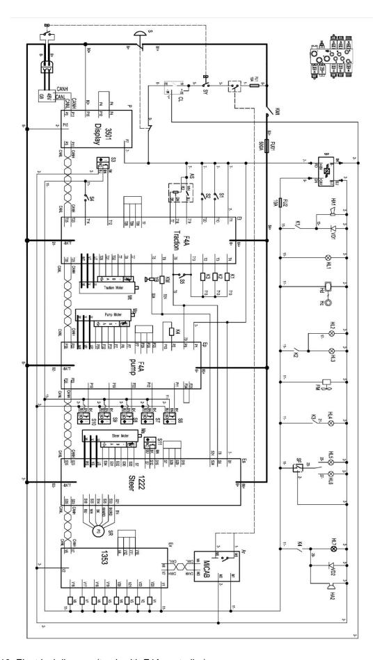
Fig. 18: Electrical diagram (truck with F4A controller)
