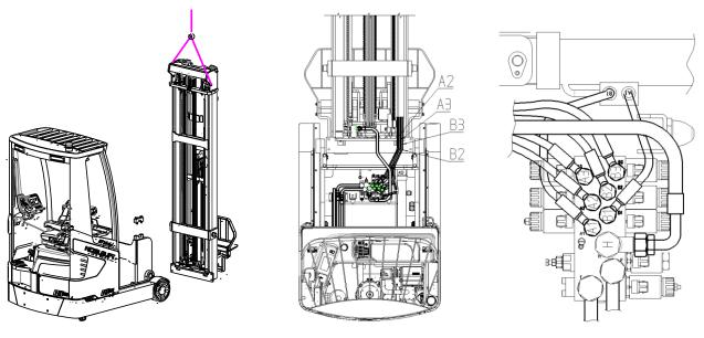
Fig 6: Mast assembling
