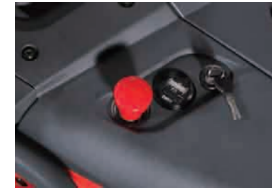
Key-switch, emergency switch and battery discharge indicator.
