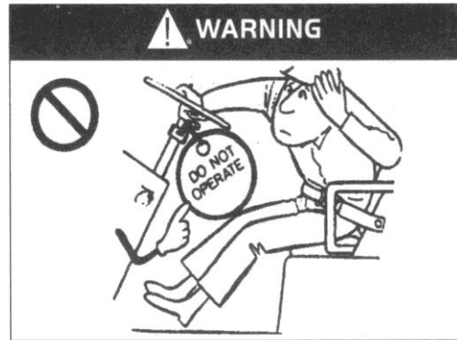
Do not drive an unsafe forklift!
